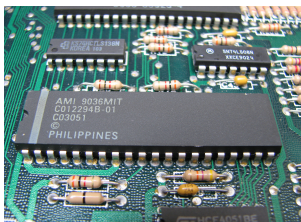
Fig.1 Original POKEY chip soldered in XE series
